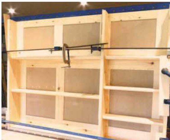
PIC 1. Where's another long clamp when you need it? With time ticking and the glue expanding, I had to act quickly. The little G clamp holds two sash cramps pinned together just enough to pull that left-hand side in tight
